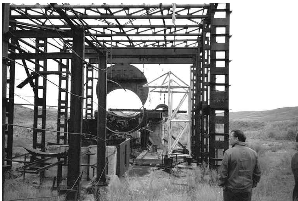
Figure 17. Structures supporting a test object (a rocket motor) outside of tunnel 169/2 at Degelen Mountain. In this experiment (4 Oct. 1989), radiation was channeled through a flexible bag filled with a special gas, and its cross-section was modified by the crescent-shaped device.
